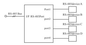
3. Serial port of master device (RS-232C) to multiple highly reliable RS-485 interface
