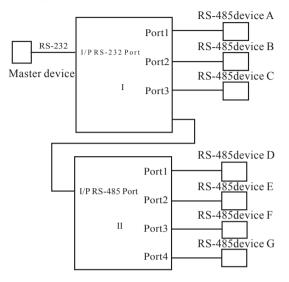
4. Extension of existing RS-485 bus to multiple highly reliable RS-485 interfaces, and maximum 128 RS-485 hubs can be connected to the RS-485 bus in parallel
