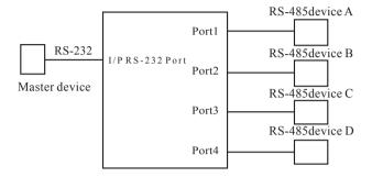
2. Extend the existing RS-485 bus to 4 highly reliable RS-485 interfaces, and maximum 128 RS-485 hubs can be connected to the RS-485 bus in parallel
